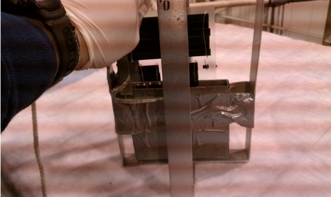
Figure 14. This figure shows the sample holder with the mounted samples being placed into the cadmium box mounted on the apparatus. The rope shown on the left side of the apparatus is used to lower the entire setup into the dry tube chamber.
