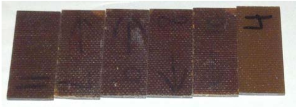
Figure 19. Photograph of the EMI-SE oriented face (MWNT ply) down. The five samples on the left are the samples that were neutron-irradiated. Sample 4 on the right was added to show the color change caused by irradiation. The numbers and arrow indicators are also visible.
