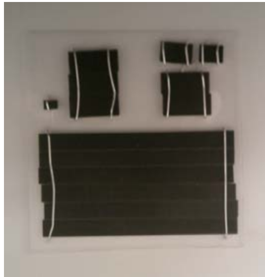
Figure 12. This figure shows the samples on the plexiglas holder with the samples wired to the holder using 0.3" diameter aluminum wire.
