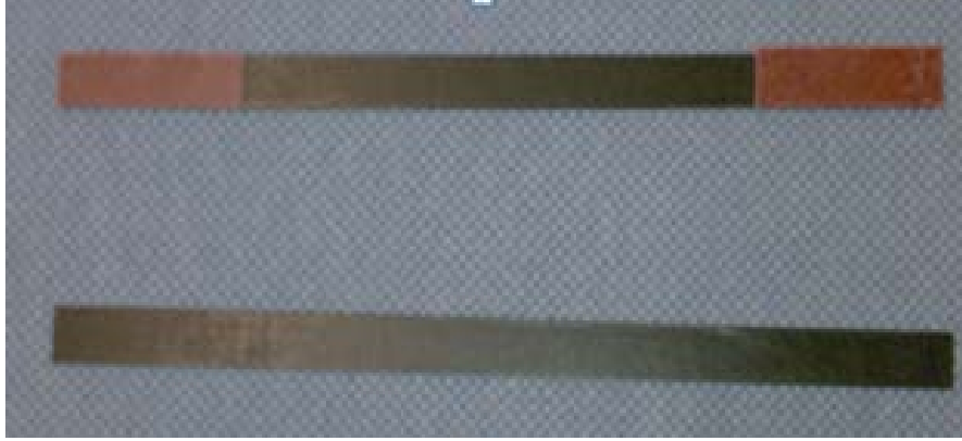
Figure 15. The upper sample shows the red tabs that have been attached to the sample for testing, as compared to the lower sample that has yet to be prepared.
