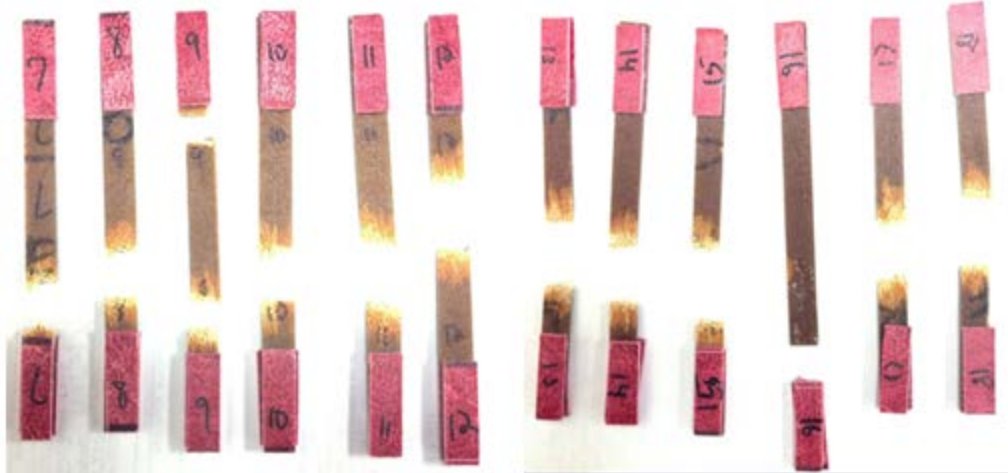
Figure 22. Photograph showing all of the samples tested to failure except for sample 16. The tabs on the bottom of sample 16 failed to remain adhered to the sample, and when the sample slipped out, it was not tested to failure. Sample 9 is unique to the sample set in that it failed in two locations simultaneously.
