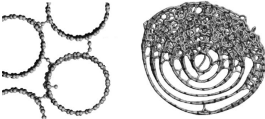
Figure 11. The image on the left shows cross-linking externally between different SWNTs. The image on the right shows cross-linking internally between concentric tubes in an MWNT. In MWNTs, cross-linking occurs internally and externally from MWNT to MWNT. Reproduced with permission from Krashenikov, et al. [34].
