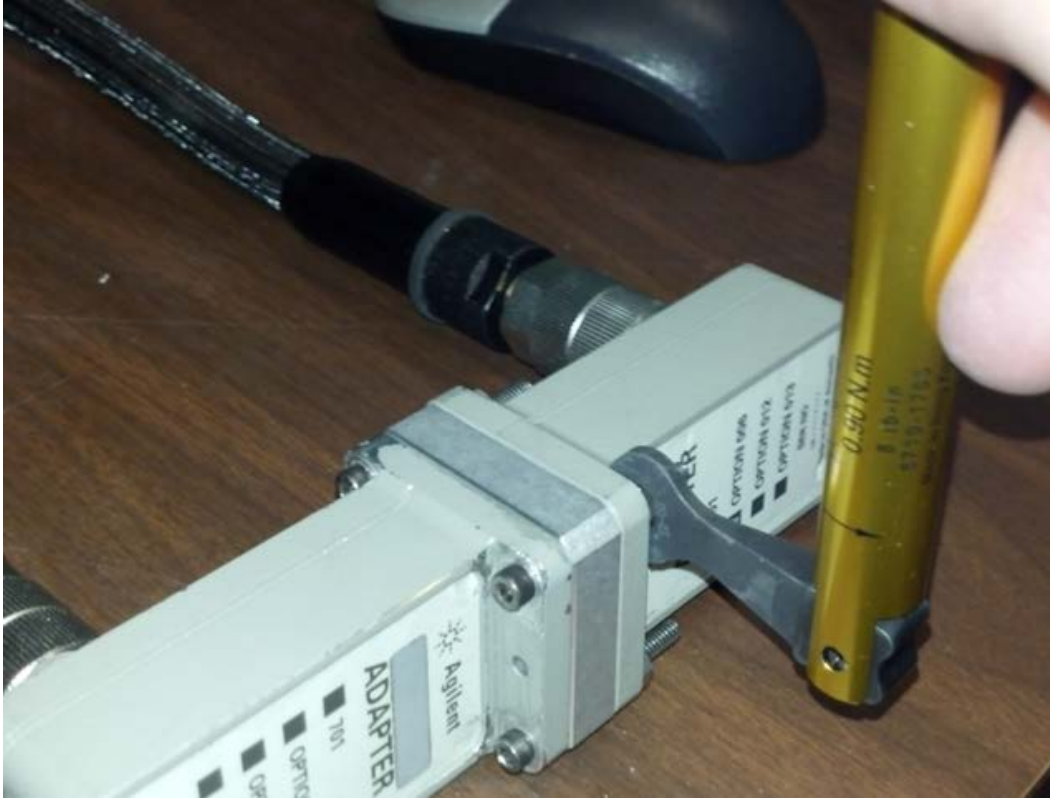
Figure 18. Photograph showing a sample being secured into the Agilent Technologies E8362B PNA Series Microwave Network Analyzer. The waveguide is secured by hex cap screws and nuts tightened to the torque specifications of the Agilent Technologies 0.9 N-m torque wrench. The left side is the port adaptor for port 1, and port 2 is on the right side of the photo.
